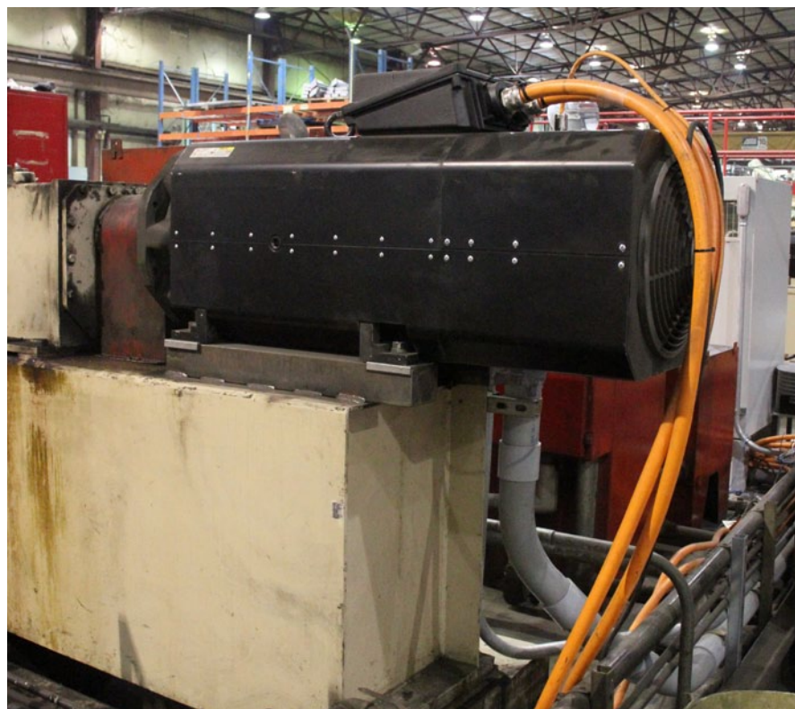
The IndraDyn MAD AC motor provides reliability and the power to feed 8-10 ton rolls of material into the machine.
