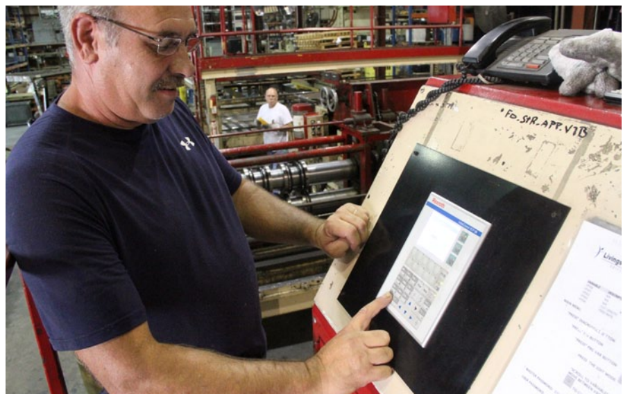
The massive metal forming machine is controlled by an intuitive HMI affording the operator more complete control and safety.
