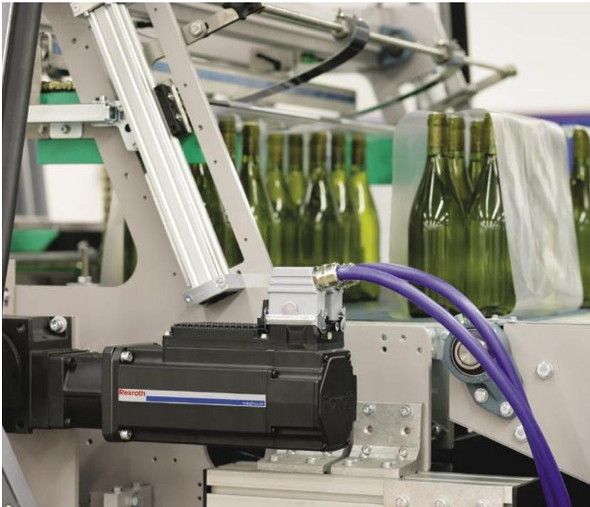
With the IndraDrive Mi, drives can be added flexibly as needed, without requiring any changes to the control cabinet.
