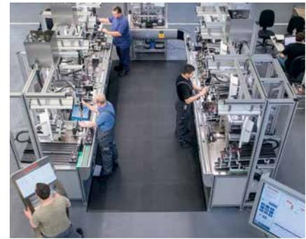
The Rexroth connected industry line allows an extensive product range to be produced without the need to perform technical or logistical setup tasks.
