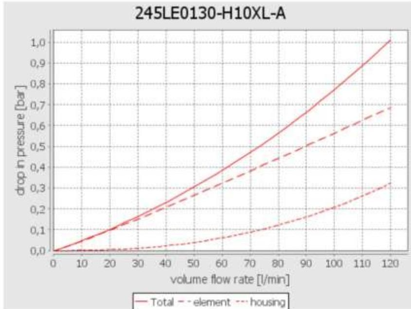
The Filter Select tool calculates pressure drop across Rexroth filters based on various user inputs
