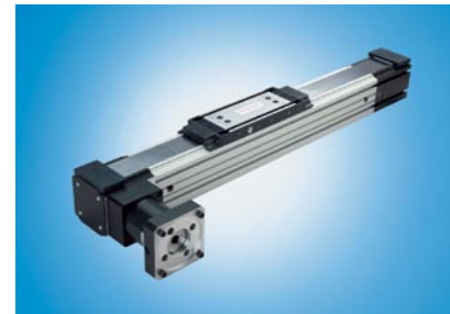
A typical belt-drive linear actuator, the Rexroth MKR, provides higher speeds and longer lengths than typical screw drive actuators. Screw drive systems offer higher precision and higher load capacities.
