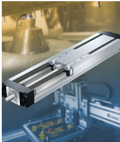
Linear motion systems combine a linear drive mechanism with a linear guide system inside a housing to create a single linear axis. Rexroth Compact Modules shown here use a precision ball screw with ball rail linear guides.
