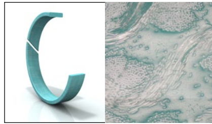
Figure 2: A composite bearing composed of polyester fabric impregnated with a polyester resin—bearing strip and cross section micrograph shown
