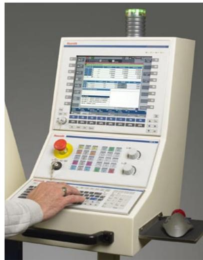
User-friendly controls built around the Rexroth IndraControl HMI reduce machine setup and changeover times.
