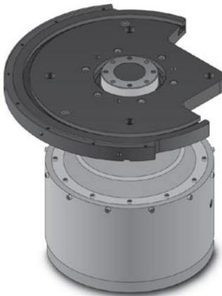
Rexroth's IndraDyn T frameless torque motor drives the Model 30's rotary, providing the most accurate radius possible in the world, repeating to an accuracy of  $\pm .077$  arc seconds with no gears or linkage to accumulate errors. The perfect radius means fewer tear-offs.
