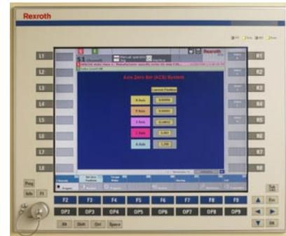
Utilities windows for setting scales or a torque meter make it easy for an operator without programming experience to maintain the grinder.
