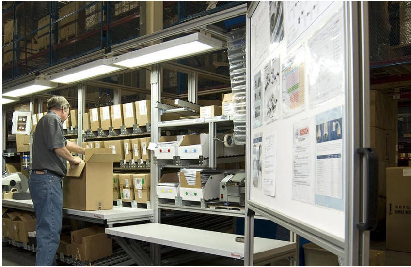
Rexroth's aluminum structural framing allowed Bosch Security Systems to add a packaging station after the initial configuration was put in place. A workstation houses brochures while a stand for bubble wrap was added to the end of the assembly line.
