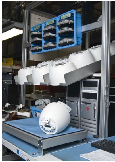
Rexroth aluminum structural framing and lean cell design keep security camera housings within reach.
