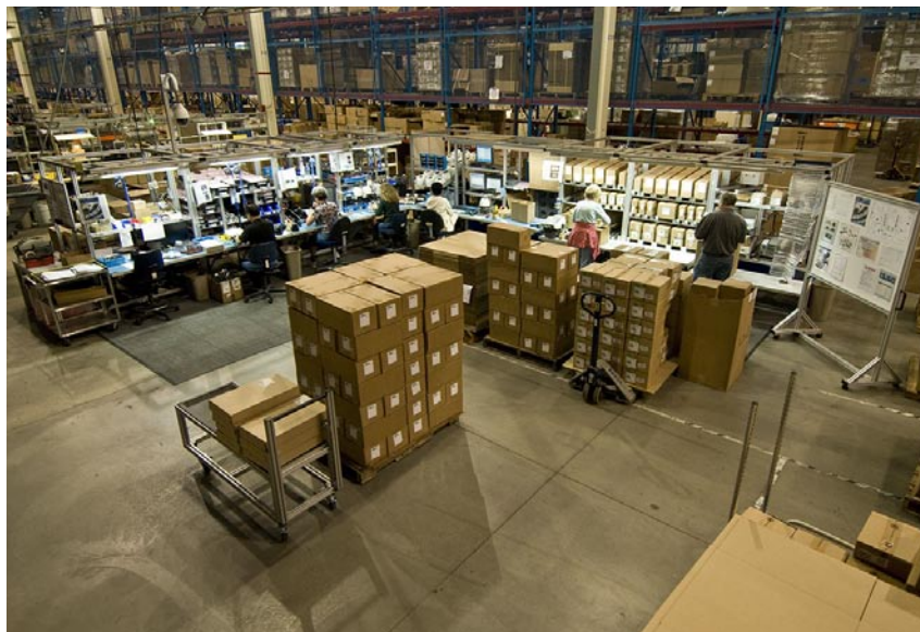
Bulk materials are stored around the perimeter of the workstations. Milkrunners maintain stock levels at each workstation.
