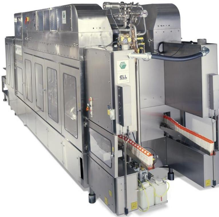
The Bosch Rexroth PPC controller and modular servo drive system provides the tight synchronization and production performance the Q-16 needs for shorter cycle dwells and higher speed timing.
