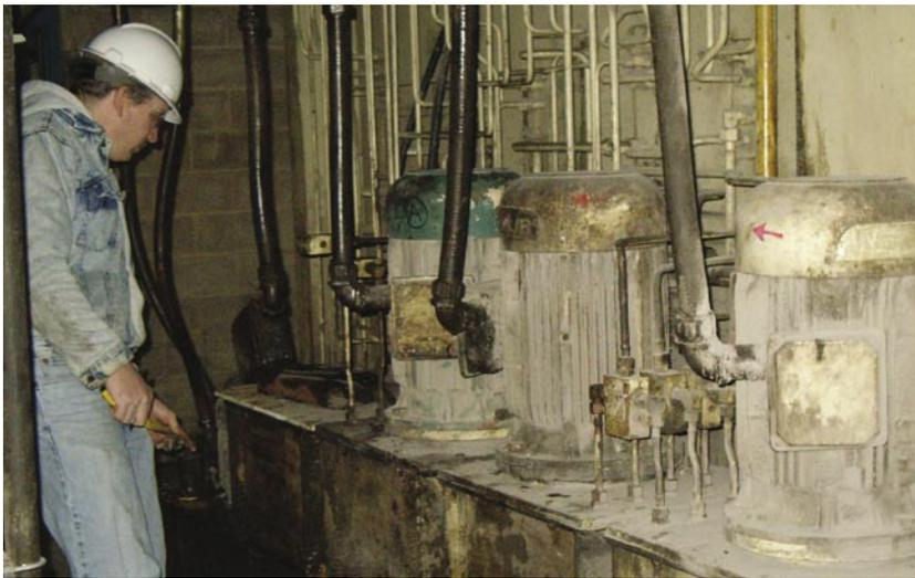
Montenay's old hydraulic system was designed in Germany and used a main power unit with gear pumps stacked together and submersed in tanks, making them difficult to access and repair.
