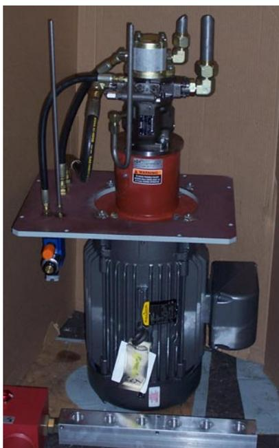
The new gear pump design has reduced the number of gear pumps to one per electric motor. Previously, six gear pumps were powered by one electric motor. (The unit will actually be positioned with the motor on top and the pump hanging down submersed in the fluid tank.)
