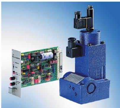
The gear pumps pass the flow through Rexroth model 2 FRE 6 proportional flow control valves, which allow an electrical signal to control the fluid flow independent of pressure and temperature variations.
