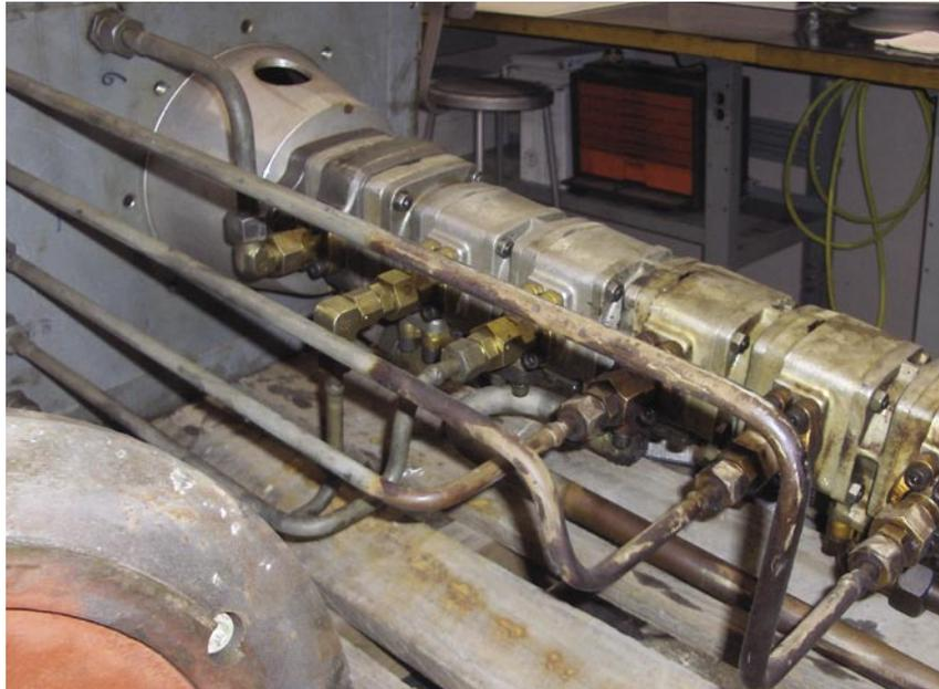
The system had 24 submersed gear pumps that set the cylinder movement rate for multiple sets of identical cylinders.
