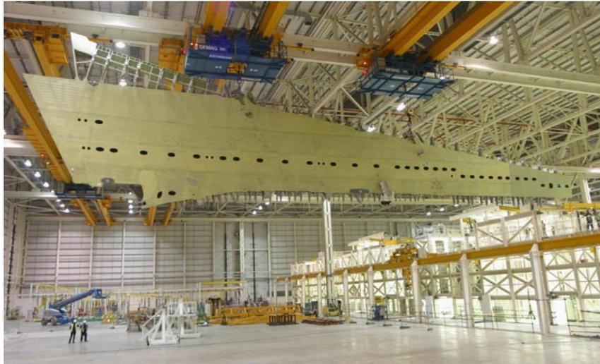
Airbus A380 wing after removal from main assembly jigs.
