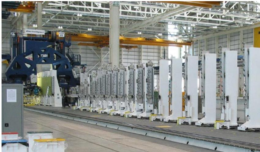
Stage 00 E4380 machine positioned over panel fixture.
