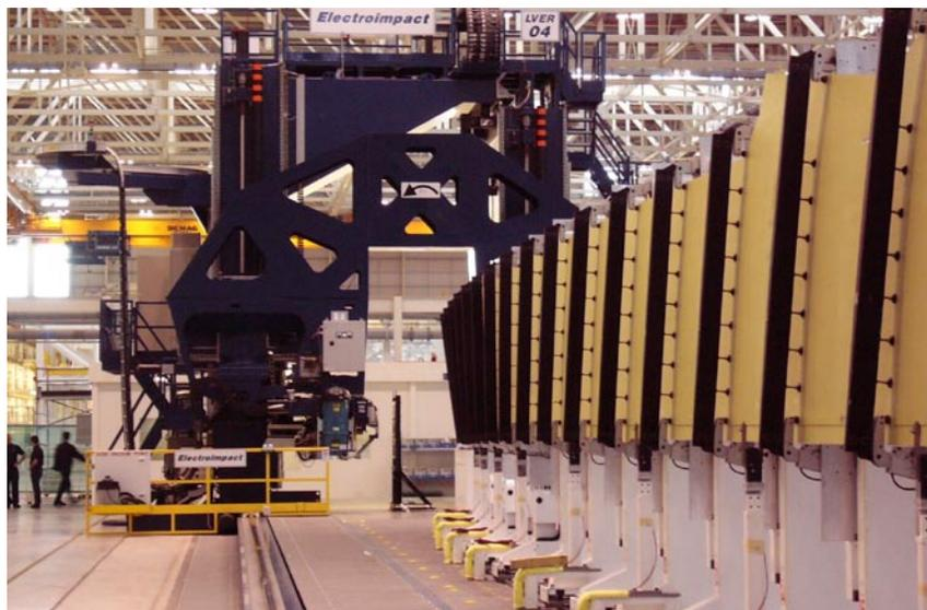
The E4380 wing panel machine attaches stringers to the skin in the Stage 00 cell.
