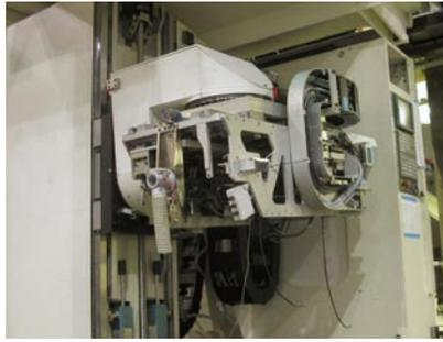
Close-up of the rotated head of the HAWDE CNC drilling machine used in Stage 01.
