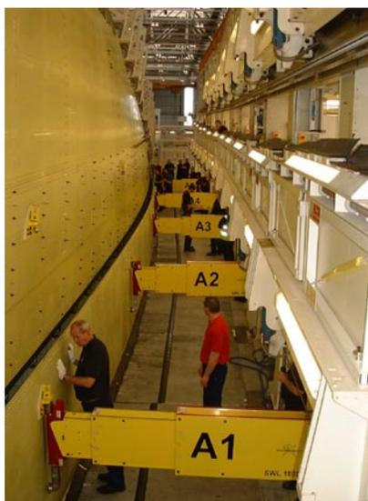
Massive, multi-arm manipulator maintains proper wing-panel shape during transfer to the Stage 01 jig.
