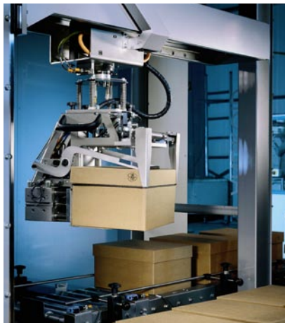
The palletizer uses six Rexroth IndraDrive servo axes with an IndraMotion for Packaging system solution.
