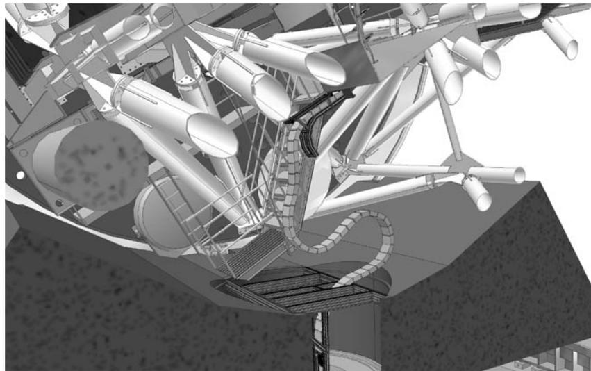
Light carrying energy chains run from the moveable mirrors high above to the stationary PEPsi below.
