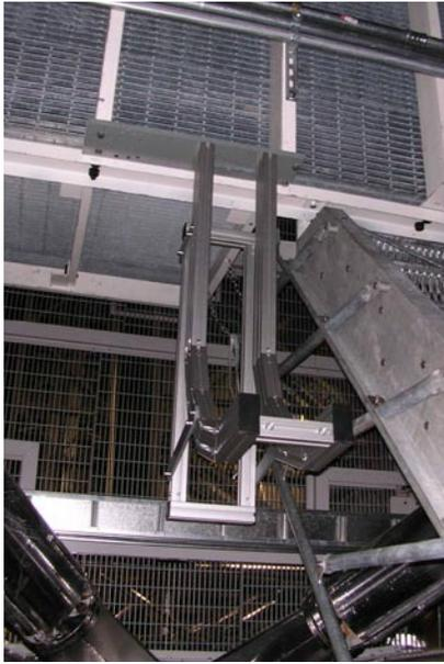
A Rexroth modular framing system will guide the energy chain, providing the strength, versatility and modularity needed to stabilize the fiber optic cables.
