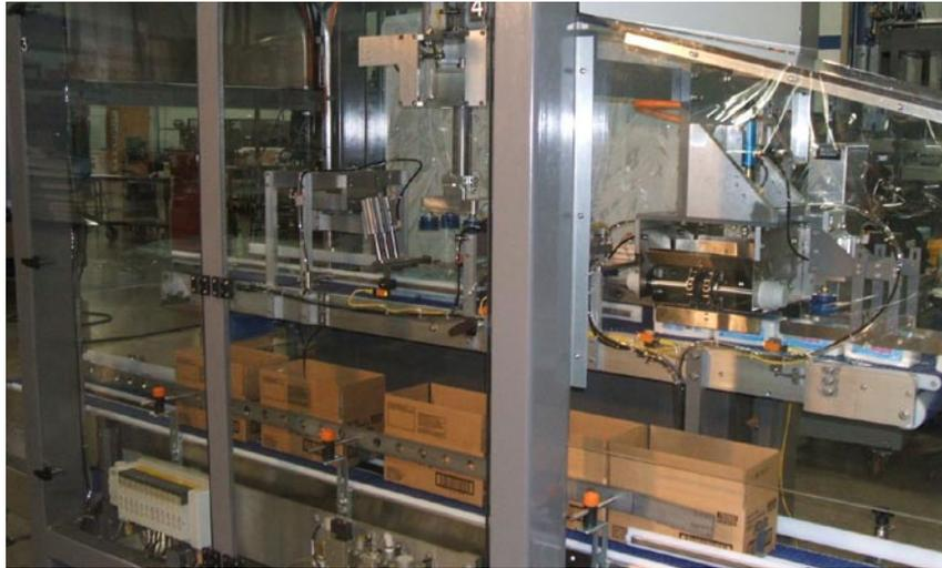
Goodman Packaging Equipment used Rexroth's IndraDrive Mi integrated servo motor/drive platform for a smaller footprint with increased flexibility and more advanced integration capabilities.
