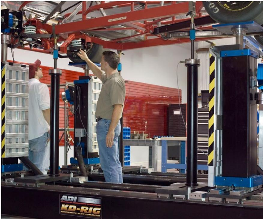
can measure such things as force over position curves: Relative to the compression of the tire, the rig can simulate and measure the forces that specific points in the suspension are experiencing. This helps the teams understand how vehicle suspensions are performing, compared to original design and engineering assumptions.
