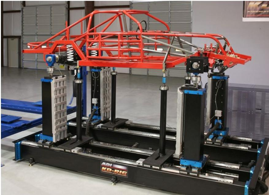
The semi-dynamic chassis and suspension testing rigs allow crews to conduct testing in a controlled environment that provides high-speed simulation data acquisition.
