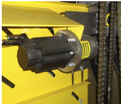
T-Tek uses Rexroth's servo motors with intelligent feedback to maintain a very high level of control for even the most delicate packaging.
