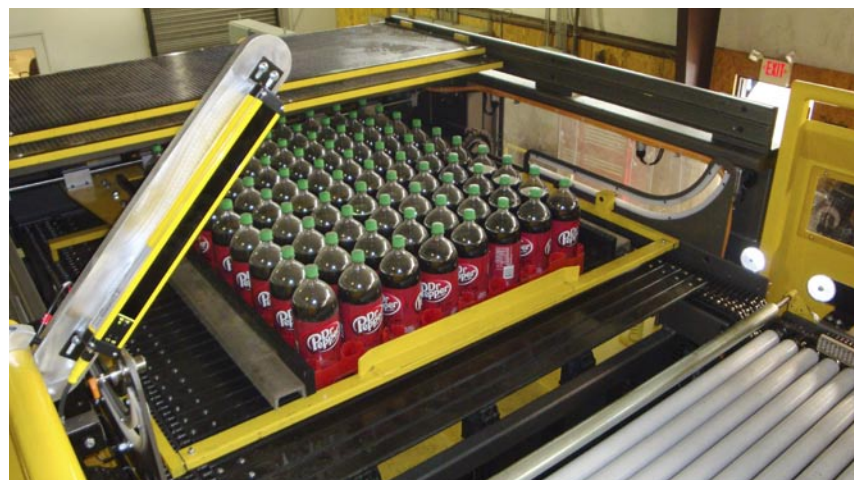
Using Rexroth's IndraDrive M drives and MSK servo motors, T-TEK saw a 15- to 20-percent improvement in apron and compression cycle times.
