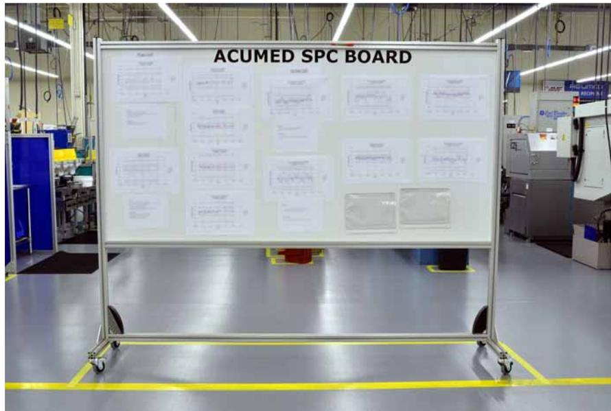
After a series of workstations were completed, remaining Rexroth structural framing was put to work in a message board that helps Acumed track projects.
