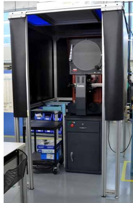
Flexibility and convenience are important advantages of Rexroth framing in creating workstations, like this unique laminar flow hood configuration.
