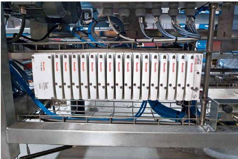
AMC uses the CL03 valve terminal system in all its packing lines and thus eliminates large control cabinets and long actuator cables.
