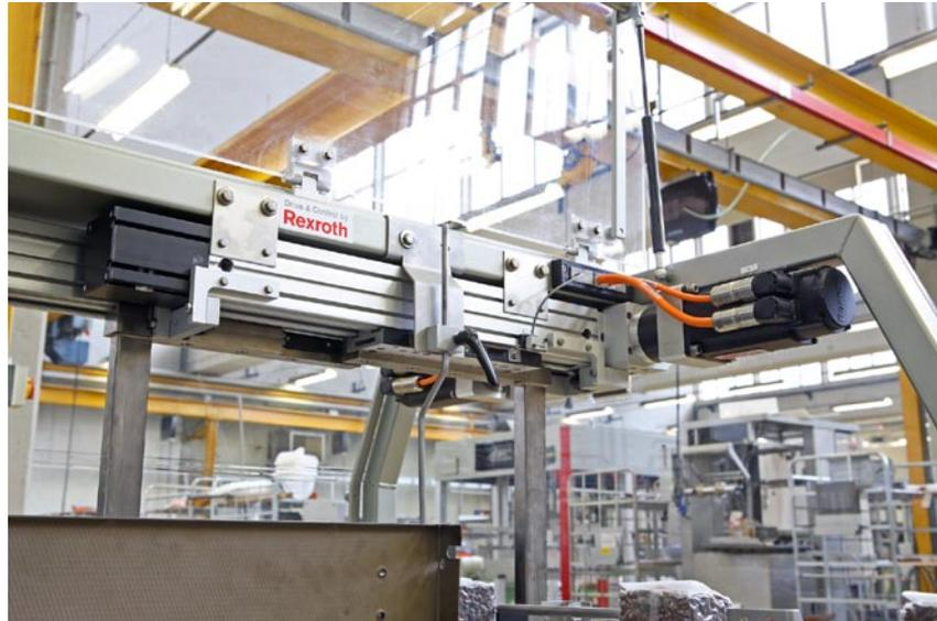
Linear modules from Rexroth's MKR series move the insertion and support plates for filling the cassette. The compact modules are combined with MSK servo drives in the CCV, making it possible for both plates to accelerate by up to 45 m/s<sup>2</sup>.
