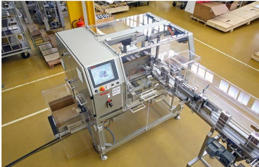
Stand-up bags are ideal for packaging solid, liquid, or powdered products and are suitable for a wide range of applications. Bosch Packaging has developed a case-packer using innovative Rexroth machine automation technology to pack the individual stand-up bags into cases.
