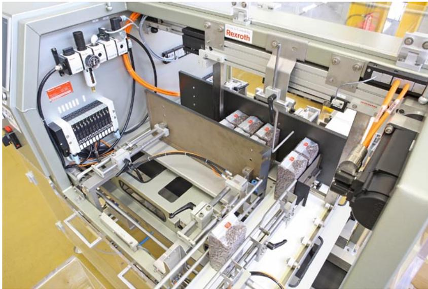
The bags are first separated, then collected and inserted in the cassette. Linear modules operate the insertion and support plates, which bring the bags exactly into position.
