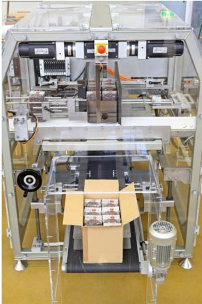
At the end of the system with innovative feed and drop technology, the filled cartons leave the case packer.
