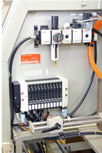
Pneumatic functions are controlled by an HF03-LG series valve unit, while the AS2 maintenance unit ensures clean compressed air.
