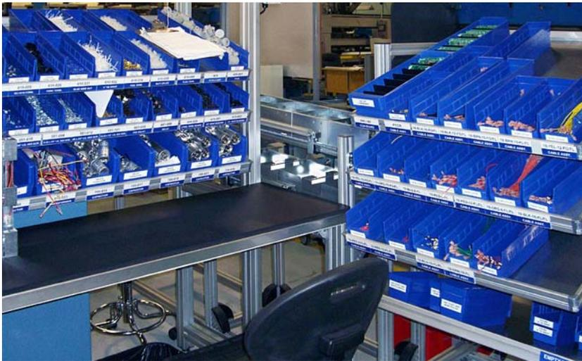
The new lean configuration has reduced work-in-progress by 40%, and FHP has gained much better control of the overall assembly process, thanks to more predictable and orderly progression of components down the line.
