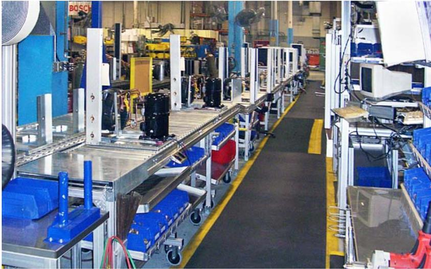
The heat pump assembly line was transformed from a batch-and-queue process into a one-piece-flow production line.
