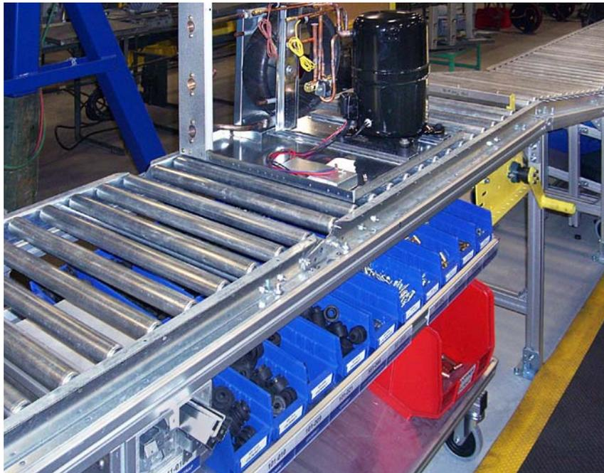
Line feeders deliver parts to the lean production line workstations on an as-needed basis.
