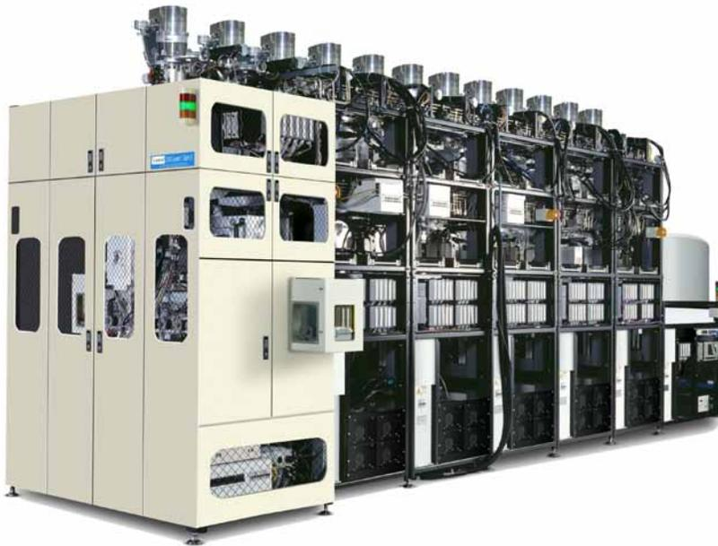
The Intevac 200 Lean<sup>®</sup> Gen II system uses a Rexroth linear motion system to increase throughput by 25% to 1,000 disks per hour.
