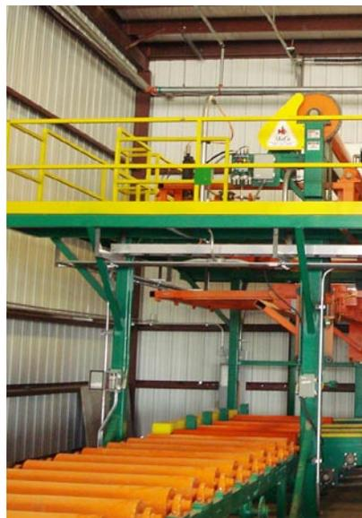
Each axis of motion follows its own onboard electronic motion profile while maintaining precise synchronization with other axes. No limit switches, time gears or external encoders are needed to determine or control axis positioning.
