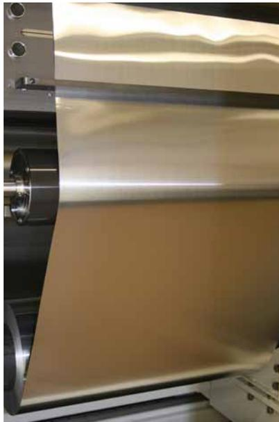
The Rexroth servomotors adjust speed to vary web tension – and use speed to vary print location. Speed and tension can be adjusted by one-percent increments as needed.
