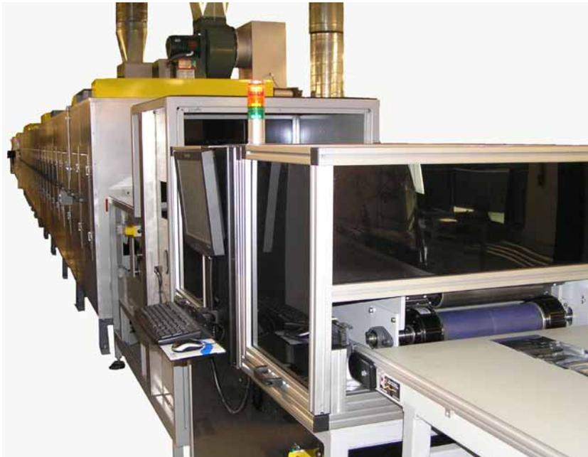
With the Rexroth SYNAX 200 system, all the machines' axes are electronically synchronized so when the line speed increases or decreases, the axes ramp up or down together to maintain precise web position.
