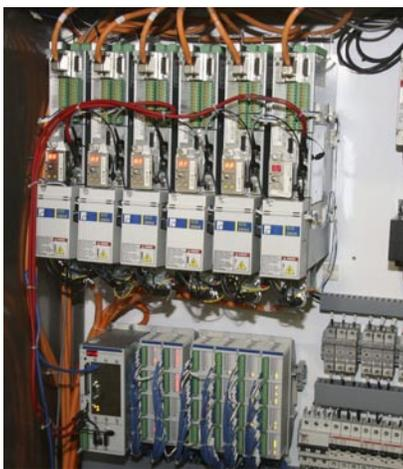
The compact design of the drive amplifiers allow the use of standard 12-inch cabinets for a smaller overall machine design.
