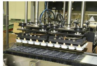
When sauce cups are being placed in the box, a separate pick head places a cardboard slip sheet in between each layer of cups to add strength and to ensure the cups are not damaged during shipment.
