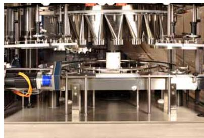
and performance, led the company to design a new servo-controlled rotary filler platform using Rexroth digital servo drives and motors.
