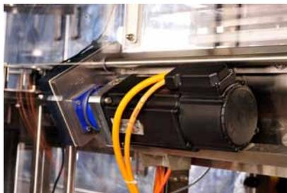
Rexroth intelligent servo drives and motors let the operator time the system's container transition between feed screw and infeed star wheel on the fly, so set up and changeover adjustments can be made with the push of a button.
