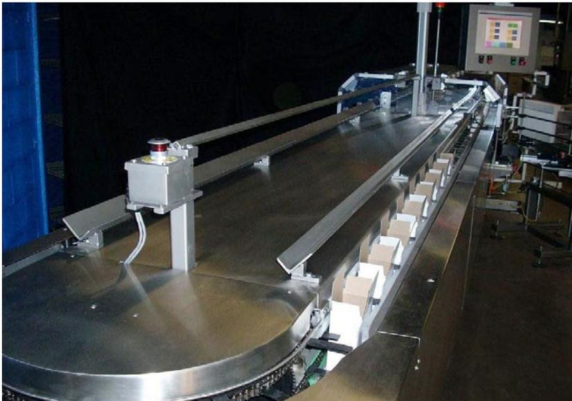
With the Rexroth drive and control system, Ultra Packaging reduced the amount of field wiring, cables, linkages and other components on its new Veronica cartoner by 60 percent while cutting their machine build time by 40 percent.
