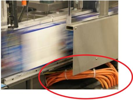
Before (above)...and after (right). The previous Veronica needed multiple cables for all the motors and drives, whereas the new design uses only a single daisy-chain cable for power and communication.
