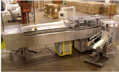
Before (above)...and after (right). The new Veronica cartoner uses a Rexroth integrated motor and drive system to improve flexibility, cut changeover time and decrease wiring and component cost.
