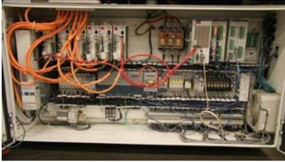
Before (left)...and after (below). Ultra Packaging used the Rexroth IndraDrive Mi system and moved the drives out of the control cabinet directly to the machine, lowering their wiring and cabinet costs in the process.
