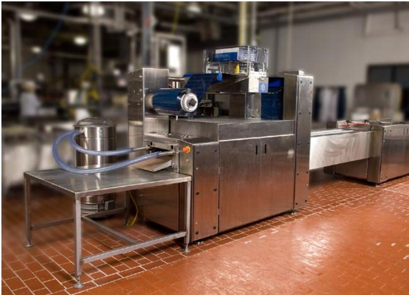
The VisionPak uses an integrated Rexroth electric drive and control, pneumatics, and linear motion platform for an ultra-sanitary and precise deli meat packaging machine.
