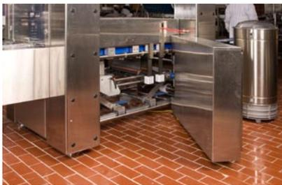
Motion and logic is controlled by a Rexroth SERCOS-based IndraMotion MLC controller with built-in motion, logic, robotic and Flex Profile capabilities—located in the unique swing-out control cabinet.
