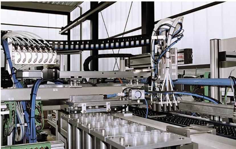
Flexibility is key: The CMS sorts the die pairs prior to the next process step.
