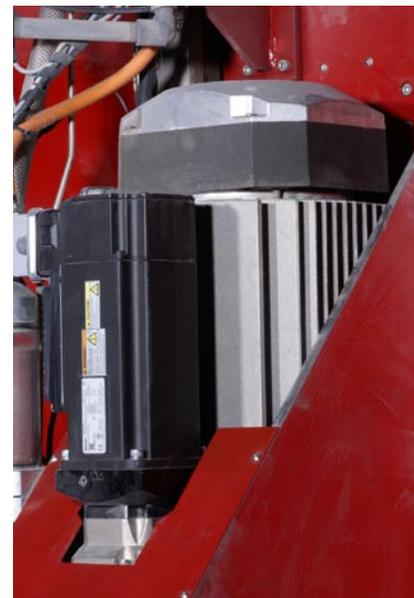
The Rexroth IndraDrive Mi combines a servomotor and drive into a single, ultracompact unit that's about 50-percent smaller than conventional servomotor and drive systems.
