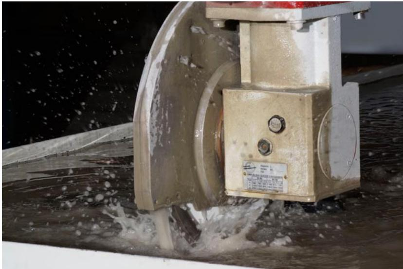
Rexroth's MTX controller precisely controls the movement of the circular saw and waterjet to make sure each piece is cut properly with minimal waste and much greater accuracy.
