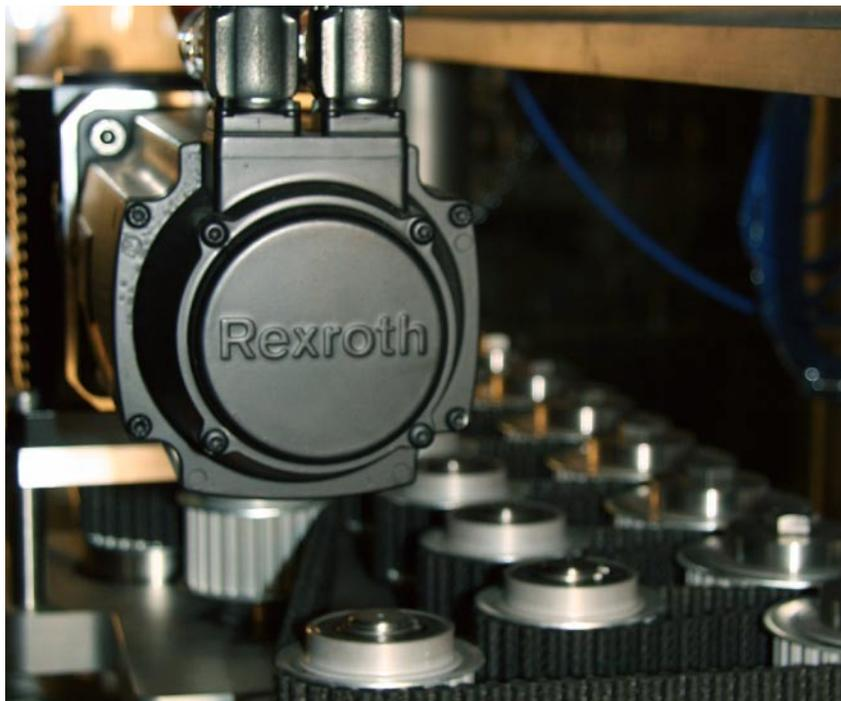
Sterilization, capping, and the transport system for bottle in- and out-feed are driven by servo controlled axes.
