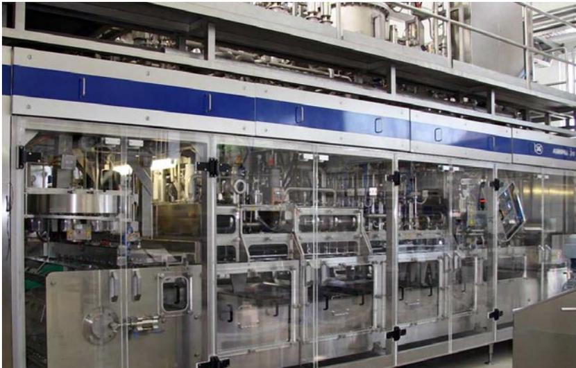
With IndraMotion for Packaging from Rexroth, the ABF 610 incorporates a compact design with an innovative machine drive concept and trendsetting safety technology.
