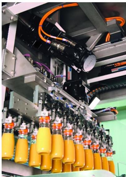
The control technology of the modular ABF 610 gives it the flexibility to fill different bottle sizes without mechanical changeovers.
