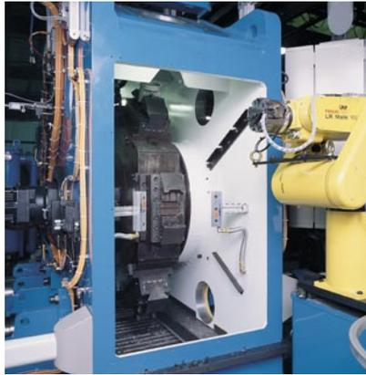
A single MTC200 CNC can command multiple machining operations involving various spindles and slide groups while coordinating automated handling and measuring systems.
