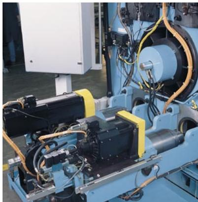
By using the SERCOS interface, the Trunnion's CNC system provides high precision and high-speed cutting as a result of velocity and position loops that are closed in the drives and independent of the network data rate.
