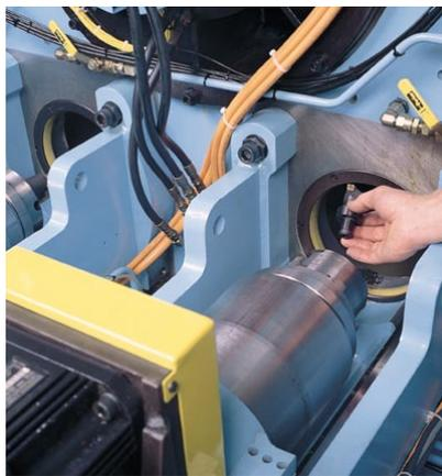
This multi-station indexing machine is similar to a dial indexing machine, except that the Trunnion has a horizontally oriented axis of rotation.
