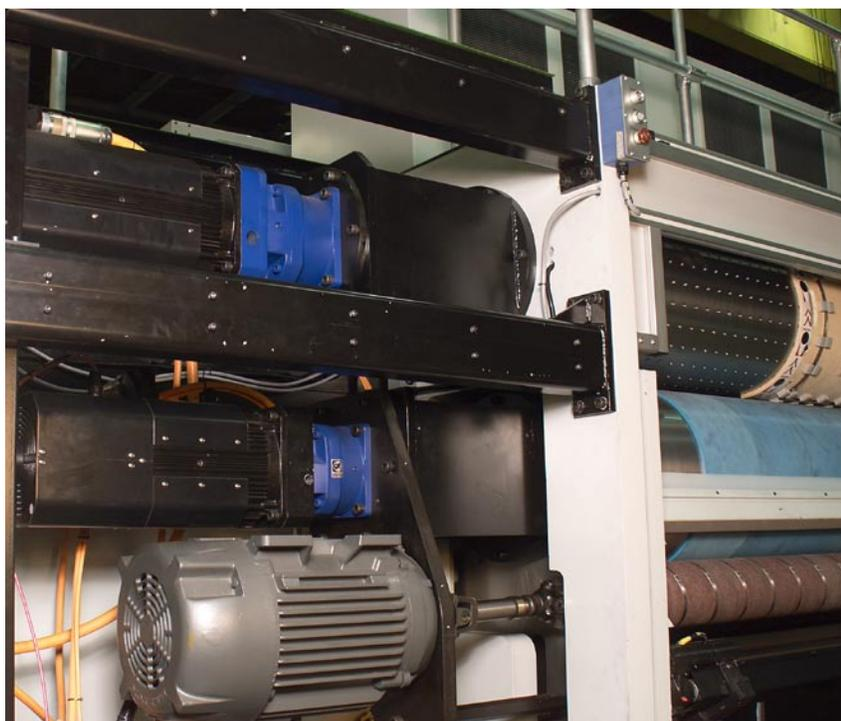
The CORRUGRAPH has an electronic line-shaft utilizing up to 37 Bosch Rexroth servo drives.
