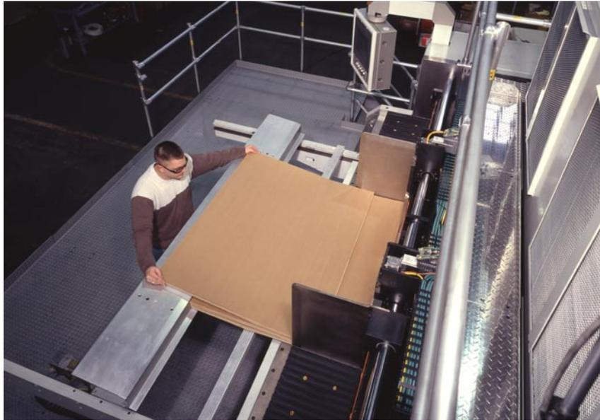
The CORRUGRAPH can produce multi-color, direct-printed graphics with die cutting in a single pass on corrugated substrates at a rated output of 10,000 sheets per hour.
