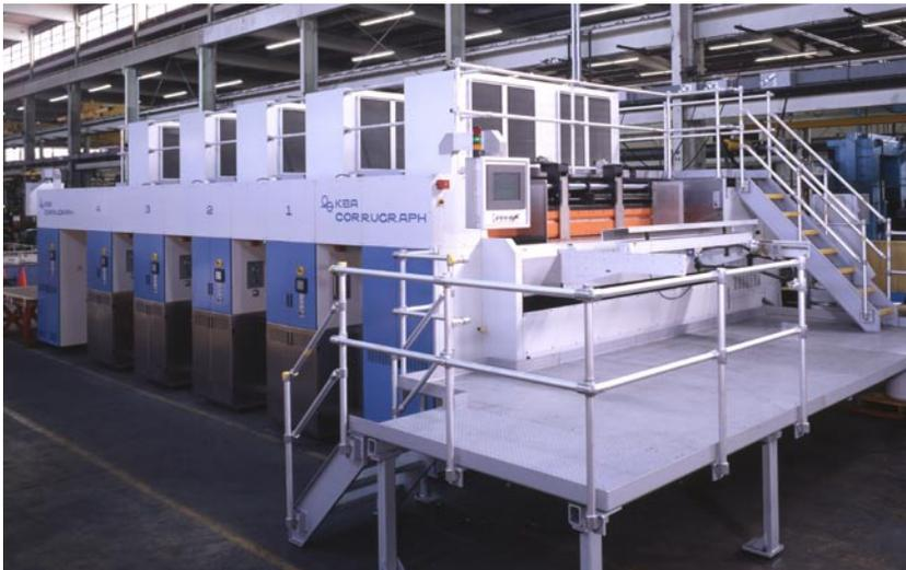
Using shaftless, gearless drive technology, KBA's CORRUGRAPH features the impression cylinders integrated in a vacuum transport system that runs the entire length of the press.
