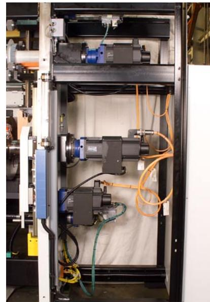
Servo drives allow the operator to change the plates, ink and/or anilox rollers in the idle units while the rest of the press is printing saleable products.
