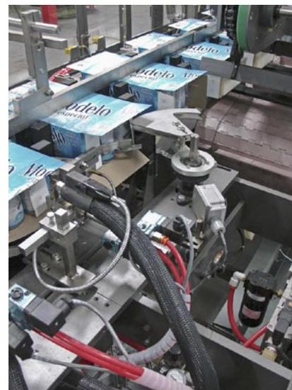
A Bosch Rexroth servo drive automatically adjusts the glue pattern and timing according to pack pattern and machine speed.
