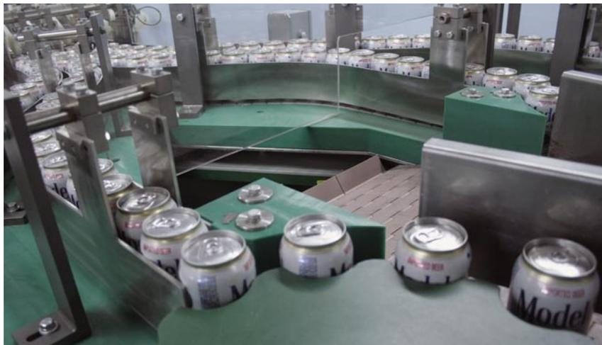
Thiele's unique servo-controlled starwheel infeed alleviates under-filled cartons, even with a low surge product at the infeed.
