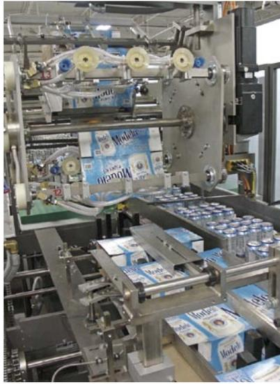
The Thiele ServoBeverage Packer incorporates a servo-driven overhead guide system, which eliminates the possibility of pack separation during the carton loading process.
