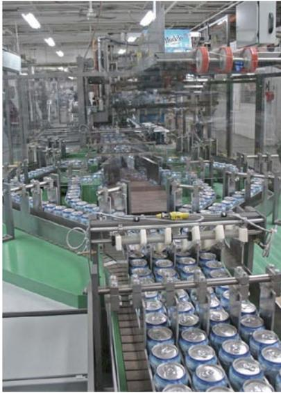
Servo axes on the Thiele ServoBeverage Packer include a rotary placer, six infeed starwheels, carton flights, barrel cam loader, and overhead confiner, all orchestrated by Bosch Rexroth servo drives and motors.
