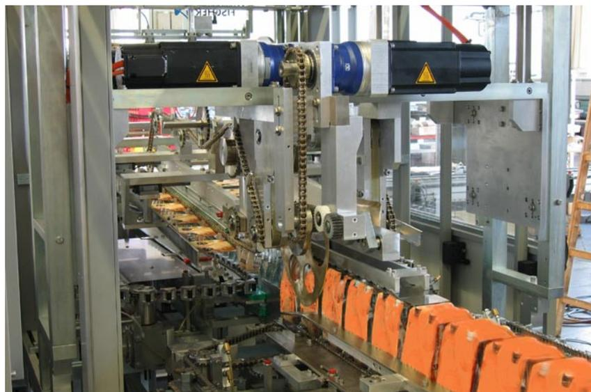
In addition to providing a safe working environment for the machine operator, the integrated "safely-reduced velocity" functionality of Rexroth's IndraDrive can also reduce downtime.
