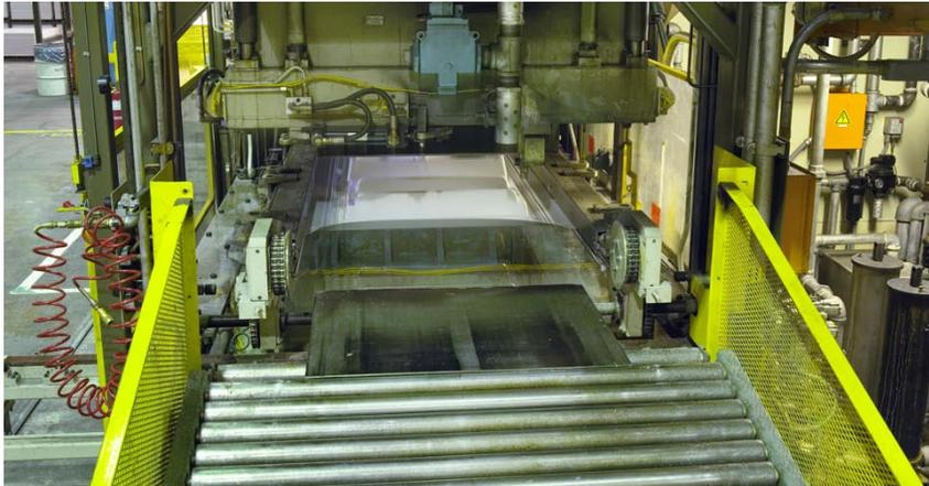
Each door liner thermoforming machine produces more than 1,000 parts per shift during three shifts per day, five days per week.
