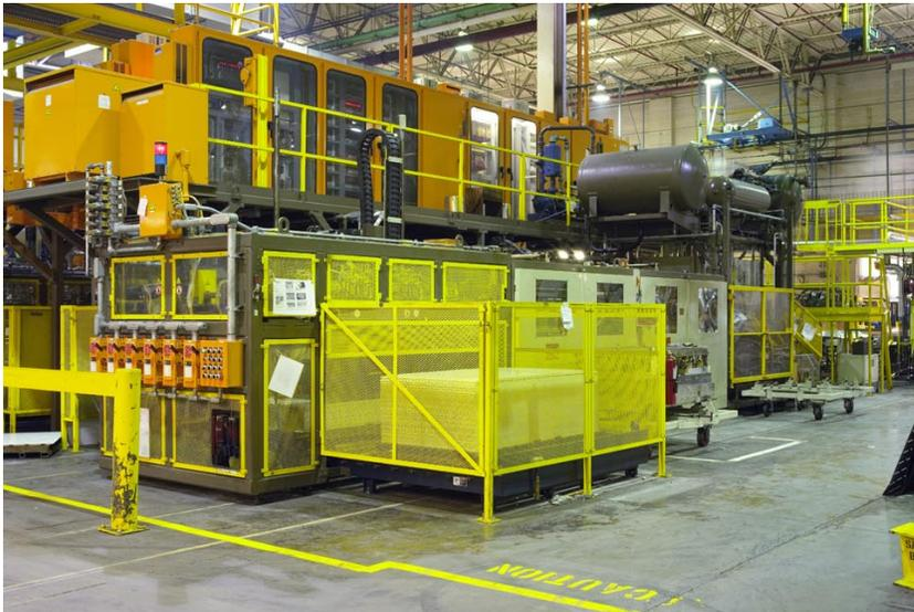
From start to finish the thermoforming process comprises the de-stacker, preheat oven, final heat oven, vacuum form press, part exit conveyor, trim press and boxing station.
