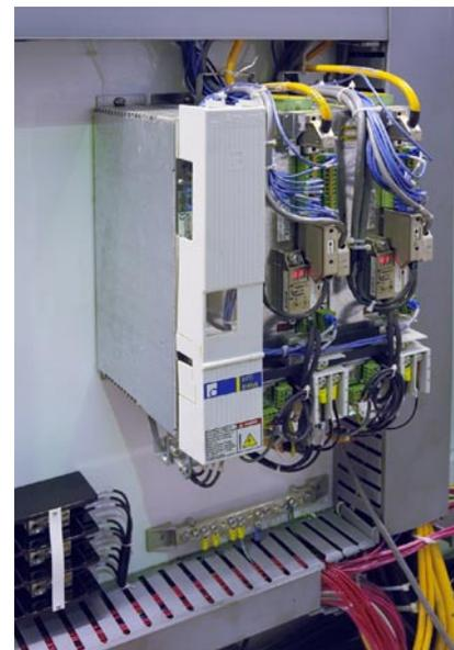
The EcoDrives used in the Whirlpool retrofit are compact, cost-effective servo drive systems for applications of 1kW up to 27kW and are especially economical for control and positioning tasks up to 27 kW.
