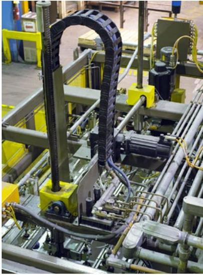
The de-stacker's drive makes eight distinct moves when picking plastic sheets from the stack, all within 20 seconds.
