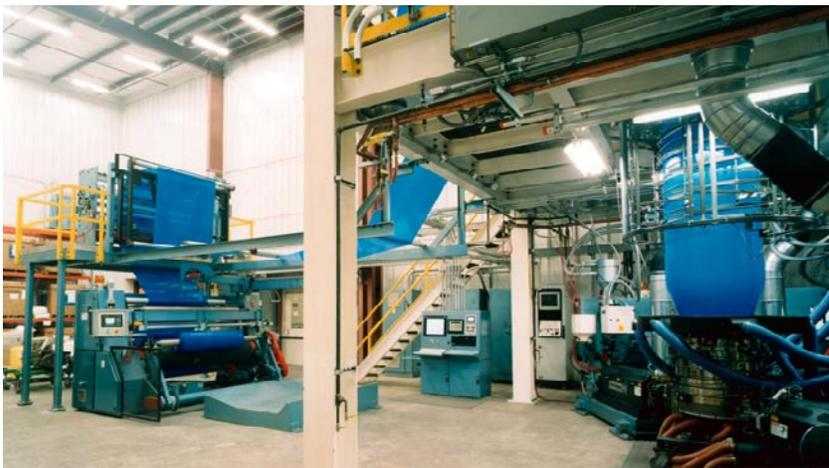
Davis Standard maintains a complete production system for in-house development and customer demonstrations, including blown film (right) and film winding (left).
