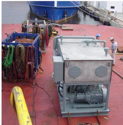
The hydraulic power unit (HPU) houses a programmable logic controller, designed to minimize field piping and wiring.
