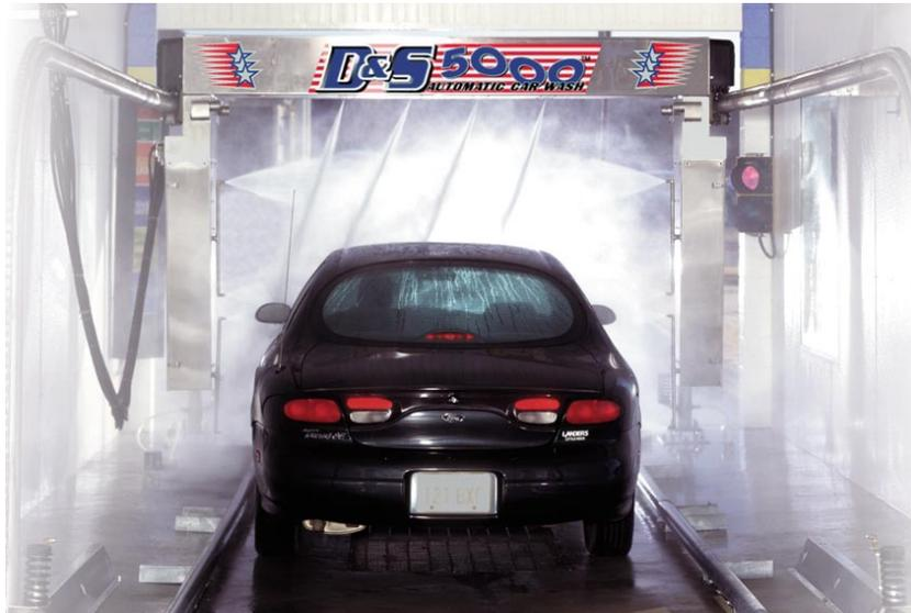
The D&S 5000™, a high-pressure touchless, brushless automatic car wash, ushered in the next generation of car wash system designs. As the gantry rounds a vehicle curve to proceed down the front or back, it reduces speed in its descent, while a hydraulic counterbalance valve prevents runaway. The gantry passes over the vehicle, applying high-pressure wash, spot-free rinse, and optional chemicals.
