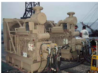
Two 750 HP diesel engine power packs were used extensively to drive four Rexroth AA10VSO140 axial piston pumps.
