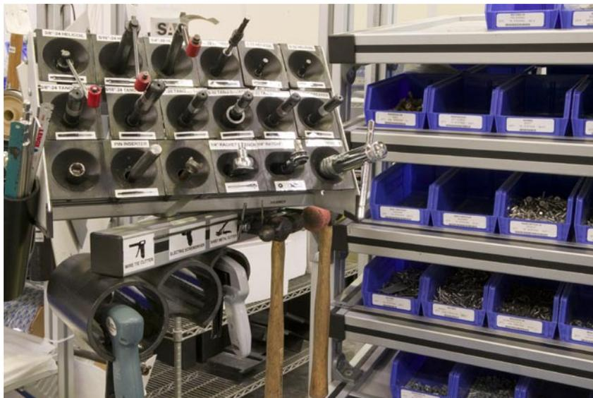
Tool holders hold all of the necessary hand tools in an ergonomic, handle-first, ready-to-use position.
