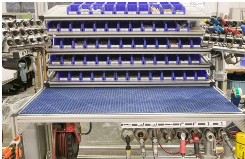
Highly customizable workstations provide timely access to the right tool at the right time. In total there are approximately 211 steps using in excess of 311 parts.
