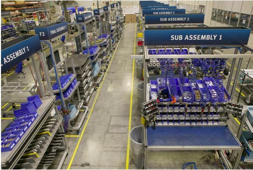
To streamline their production line, C & D Zodiac now employs station carts made of Rexroth's aluminum structural framing to transport airline seats from station to station. Converting to a continuous flow line has led C & D to nearly a 200% increase in airline seat production.
