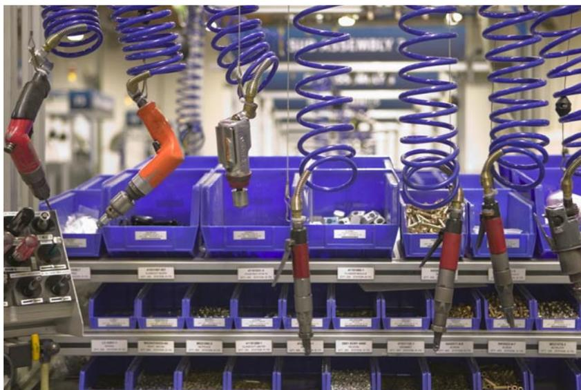
Complete with air lines that descend from the top of the workbench, overhead balancers occupy the final stations.
