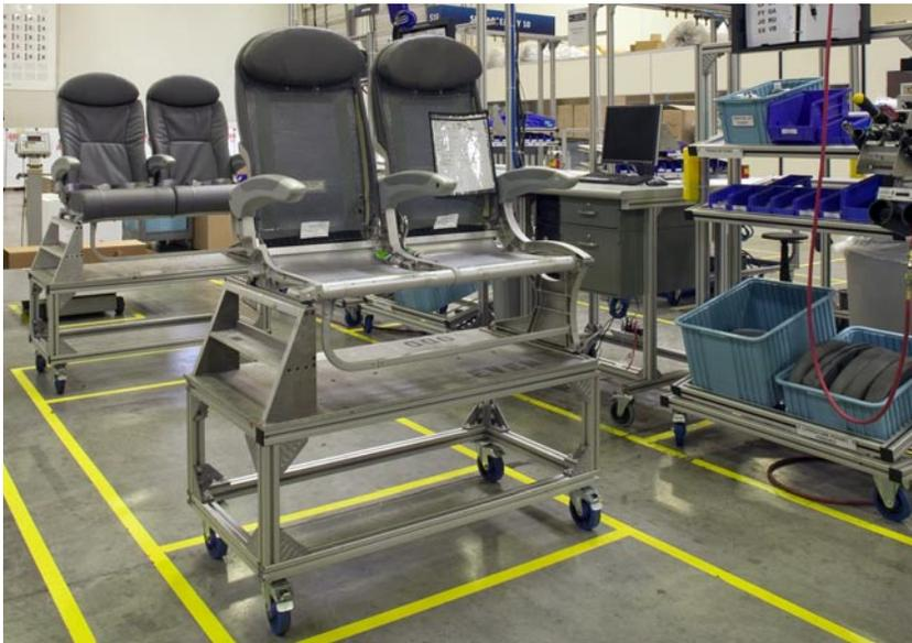
The cart moves down the production line from station to station where sub-assemblies are installed onto the seat.
