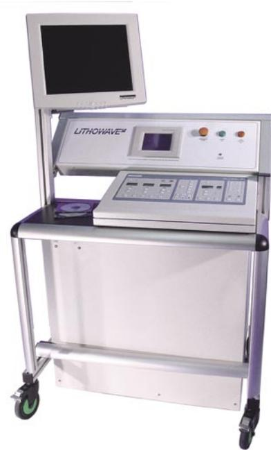
Rexroth aluminum extrusions were used for the Lithowave’s control cart, as well as in the main structure of the lithotripter itself.
