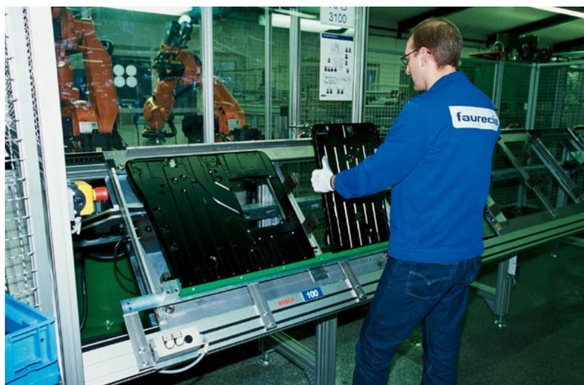
The seats’ metal structures, which are placed on the pallets, weigh approximately 88 pounds, thus the angle of the pallets offers workers needed support to prevent back injuries.
