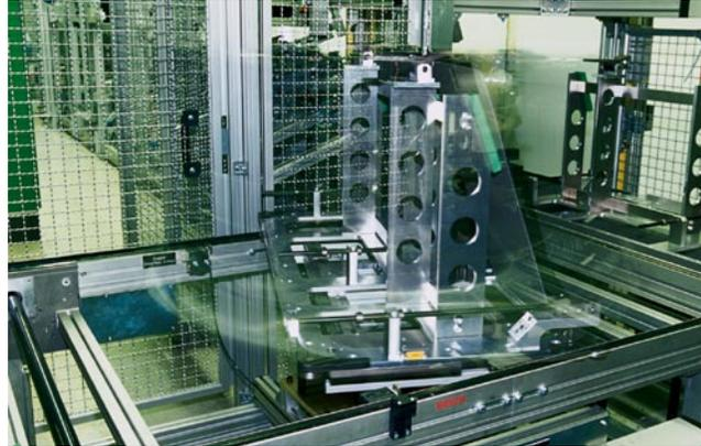
(Left) Because the system areas containing automatic stations such as robots are enclosed by a Rexroth protective fence, "accidental" entry into these areas is impossible. (Right) The pallets are rotated by 180 degrees on a lift-rotate unit prior to further processing.
