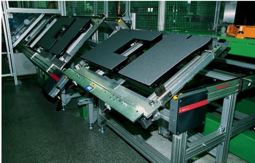
Ergonomics were a key consideration in designing the *TS4plus* transfer system to accommodate workpiece pallets at a 45-degree angle.
