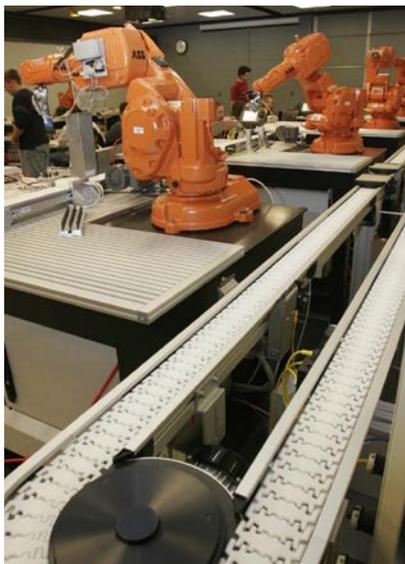
The VarioFlow single-strand flexible chain conveyor provides students with options to manage virtually any material handling requirement.
