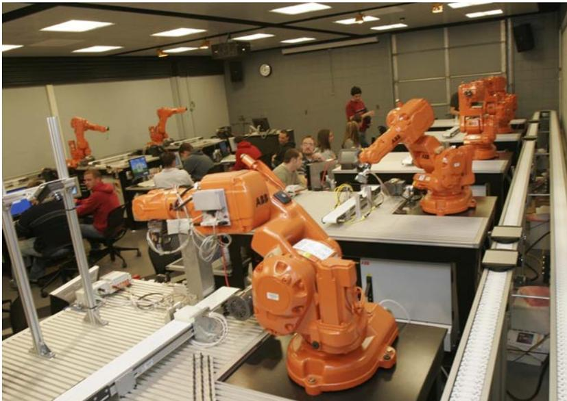
Bosch Rexroth VarioFlow flexible conveyors allow students to connect the individual workstations with one another to integrate complete multi-step assembly tasks.
