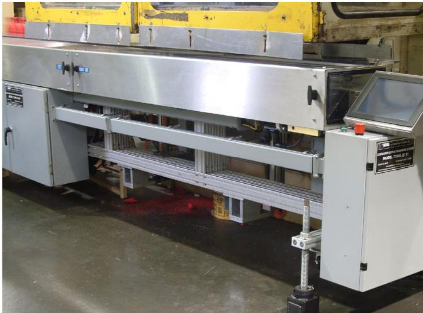
KASS switched from welded structural steel framing on its extrusion shuttle blowmolder takeout systems to Rexroth's extruded aluminum framing, cutting time and saving money on machine assembly.
