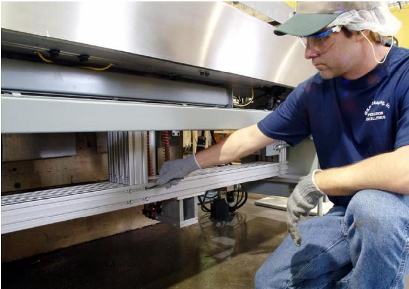
The bolt-together construction of the Rexroth aluminum framing line reduced the build time for KASS machine frames from weeks to days compared to using welded steel.
