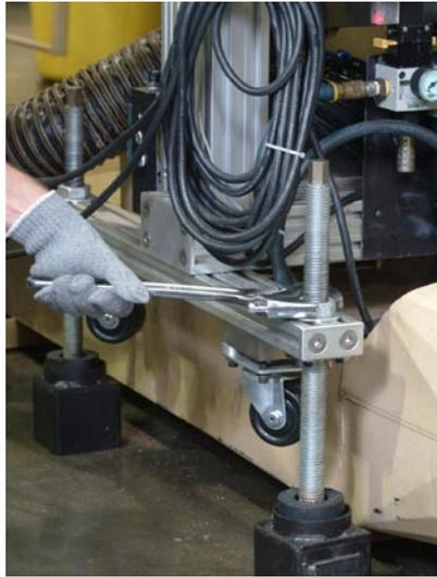
Screw-type legs allow six inches of height adjustment for alignment with other downline equipment, while the rigid Rexroth framing and connector system provides superior vibration resistance.
