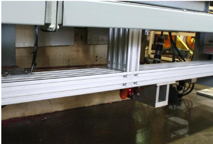
The Rexroth extruded aluminum framing proved its durability and alleviated concerns from KASS about machine vibration and shock to the frame from repetitive motion.
