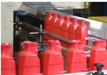
The T200E can handle containers from five inches to 12 inches in height and depths from 1.25 inches to six inches.
