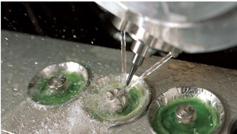
Milling of an occlusal surface of a titanium crown in a KaVo Everest® engine.
