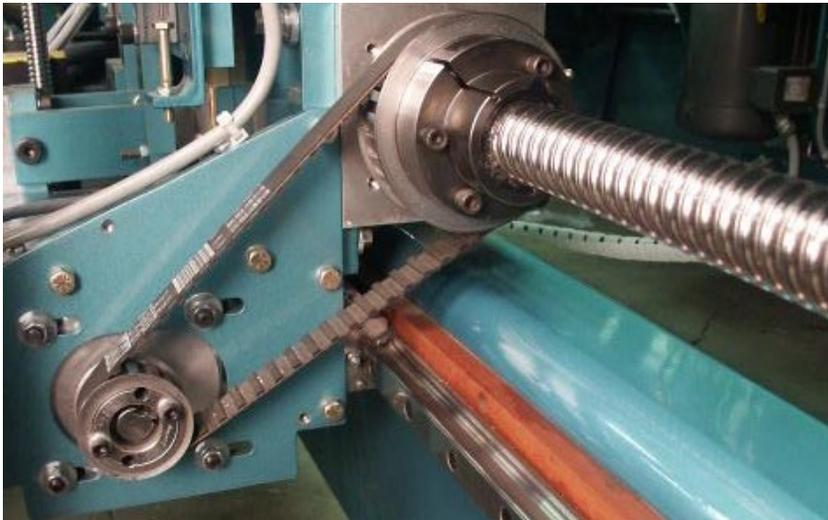
The geometrical design and extremely smooth surface finish of the Rexroth raceway results in lower friction during ball recirculation.
