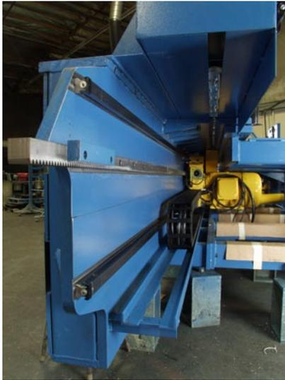
Rexroth Ball Rail linear guides support the saw assembly both vertically and horizontally to provide extreme stability and to maintain a squareness of  $\pm 0.0005$  inch, thereby achieving a surface finish as fine as 32 micro inches.
