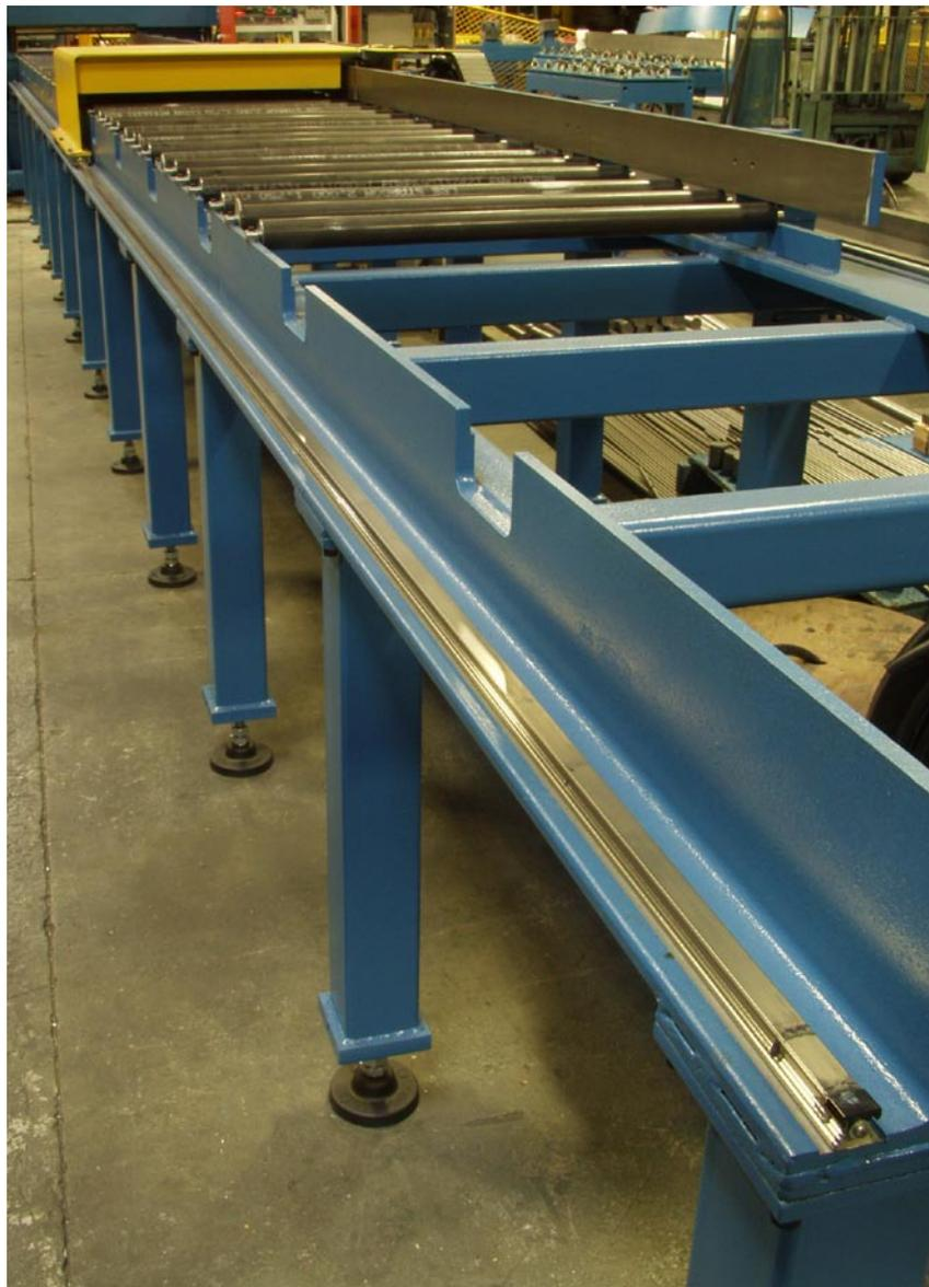
Rexroth Ball Rail linear guides equipped with RailSeal™ cover strips are used to advance metal into the sawing area. The patented rail cover reduces installation time and contamination failures, and simplifies the replacement of damaged rails.
