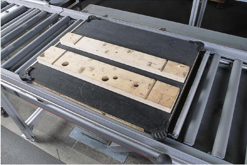
Pfannenberg continues to use simple chip board carriers as workpiece pallets in the Rexroth EcoFlow linking system. Plastic corners act as spacers and prevent employees from getting their fingers caught between two workpiece pallets.
