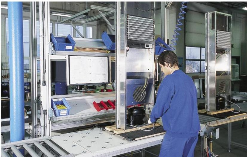
Everything in the right place: boards with work information explain the assembly steps, all the parts required are within easy reach, and the tools are ready at hand. In addition, the ball rollers recessed in the table top make it easier to turn the workpiece pallet.
