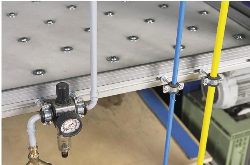
The T-groove means supply lines can be installed quickly and neatly, providing every workplace with power and compressed air for the appropriate tools.
