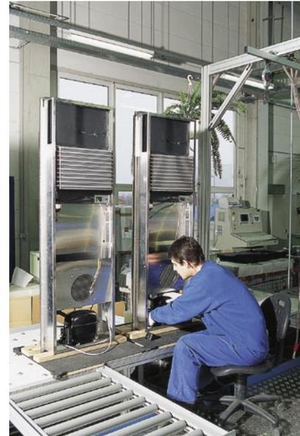
(Left) The combination of linking elements with rollers and work tables with recessed ball rollers enables different system layouts. Thanks to this design, it was easy for Pfannenberg to retrofit an additional workplace with test station. (Right) The platform is a simple, but ingenious solution for this workplace. Instead of always standing during work, sometimes even on a ladder for particularly high cooling units, the employees can now work here sitting and standing.
