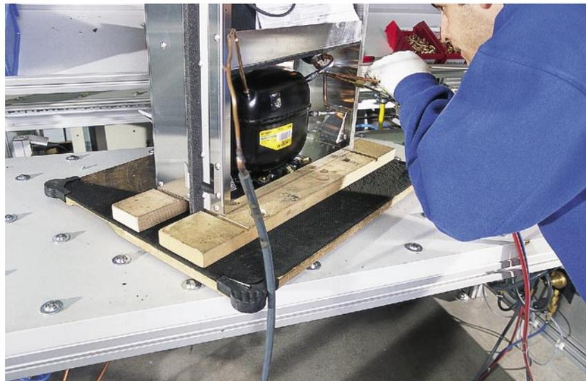
Ball rollers recessed in the table top make it easier to turn the workpiece pallets at the workplace.
