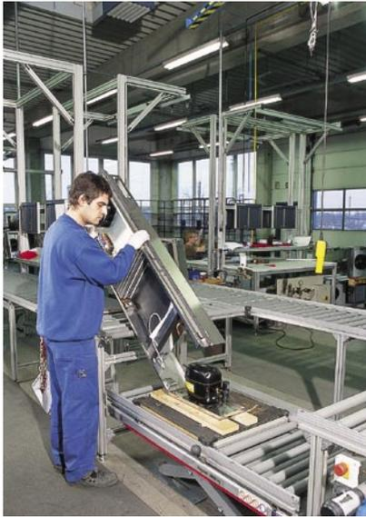
It is now easy for the employees to set up cooling units of up to 75 kg weight by simply rolling them off the EcoFlow linking system onto the lowered adjustable table.
