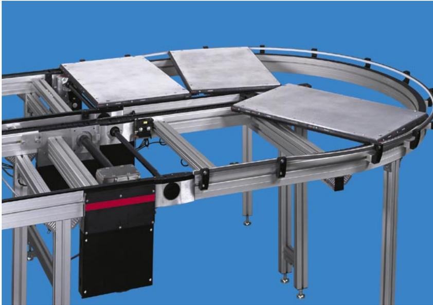
Bosch Rexroth TS2plus Flexible Transfer System
