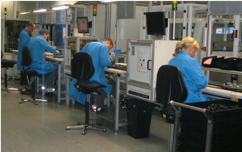
By installing the TS2plus Flexible Transfer System and IndraControl VSP 40 HMI controller, Schrader increased tire sensor production from 3 million to 5 million units per year.
