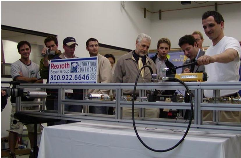
The "tug-of-war" tether pull machine allows two samples to be tested simultaneously in order to determine a winner.
