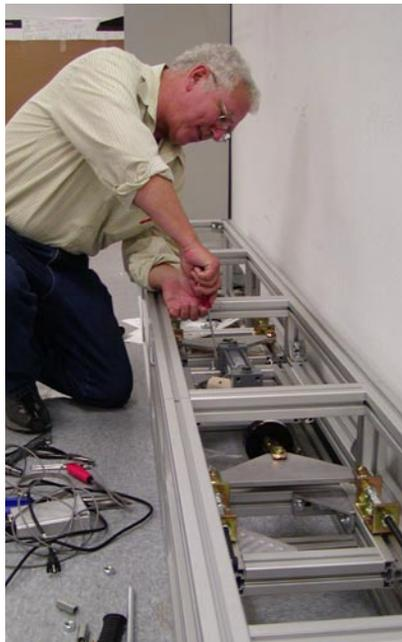
Every aluminum structural framing component is reusable, making it simple for the team to adapt the machine as design needs develop and change.
